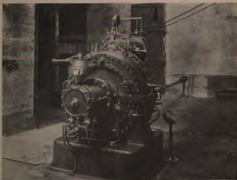
FIG. 83.—The Armengaud and Lemale gas turbine. This view and the preceding one show the wheel casing, governor, and general arrangement.
